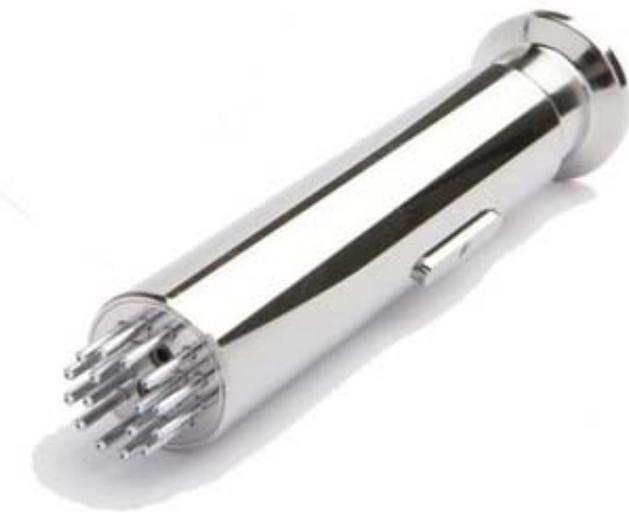
To increase tablet output, we suggested the use of multi-tips. Trials were conducted using multi-two tooling (a tool with two tips). During this test period, tablet output was increased to more than 1 million tablets per hour, with the press running at a speed of 60% capacity. The result was a 66% increase in productivity.
