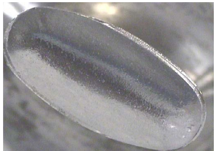
FIGURE 1: HPG-S punch after producing 4.5 million tablets, showing significant wear across the whole punch tip face and tip straight.
