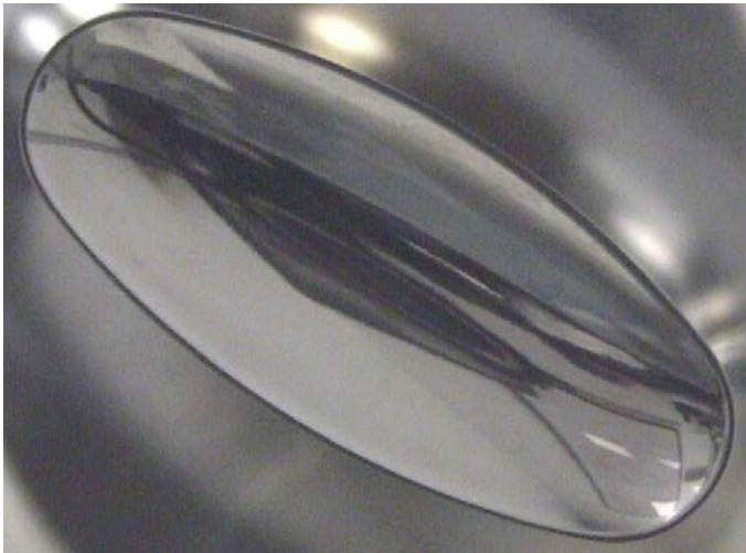
FIGURE 2: RS coated punch these were removed after producing 35 million tablets .
